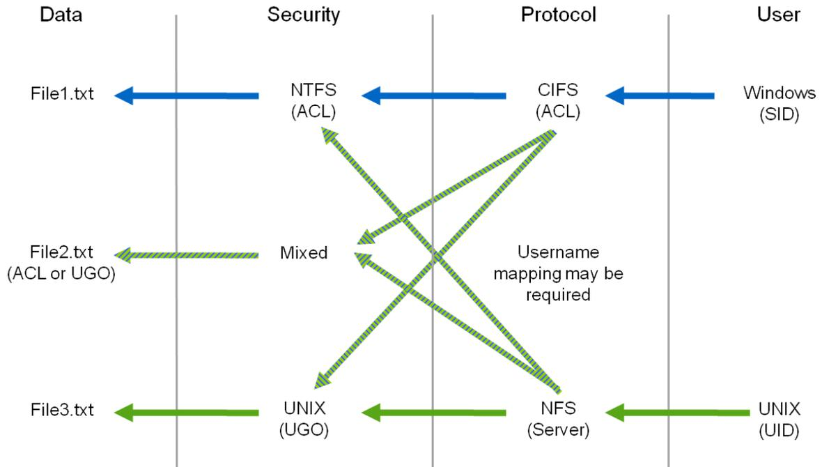
**FIGURE 13: MULTIPROTOCOL ACCESS AND USER-NAME MAPPING**
