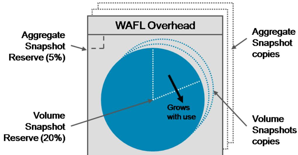
**FIGURE 17: AGGREGATE AND VOLUME SNAPSHOT RESERVES**
