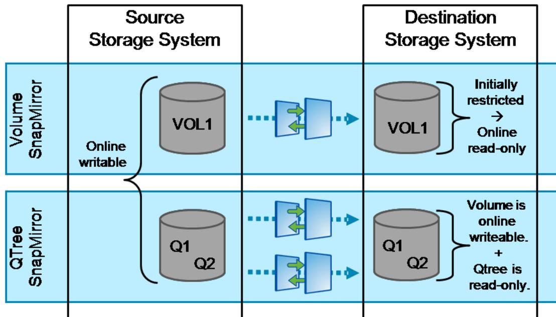
**FIGURE 18 :SNAPMIRROR VOLUME AND QTREE CONFIGURATION**
