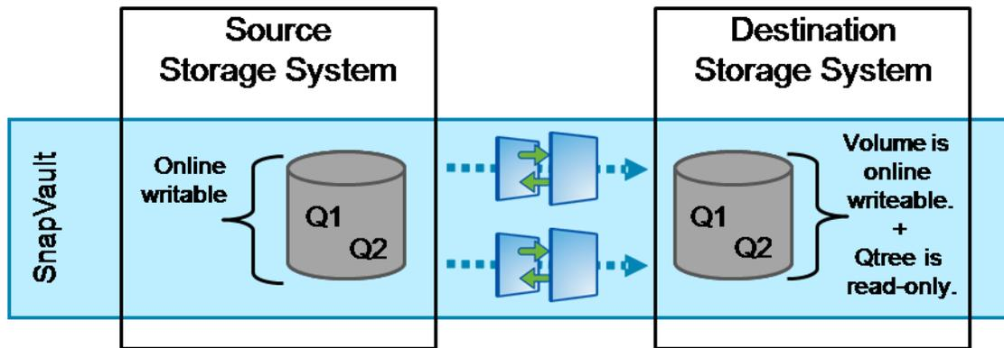
**FIGURE 22: SNAPVAULT VOLUME AND QTREE CONFIGURATION**
