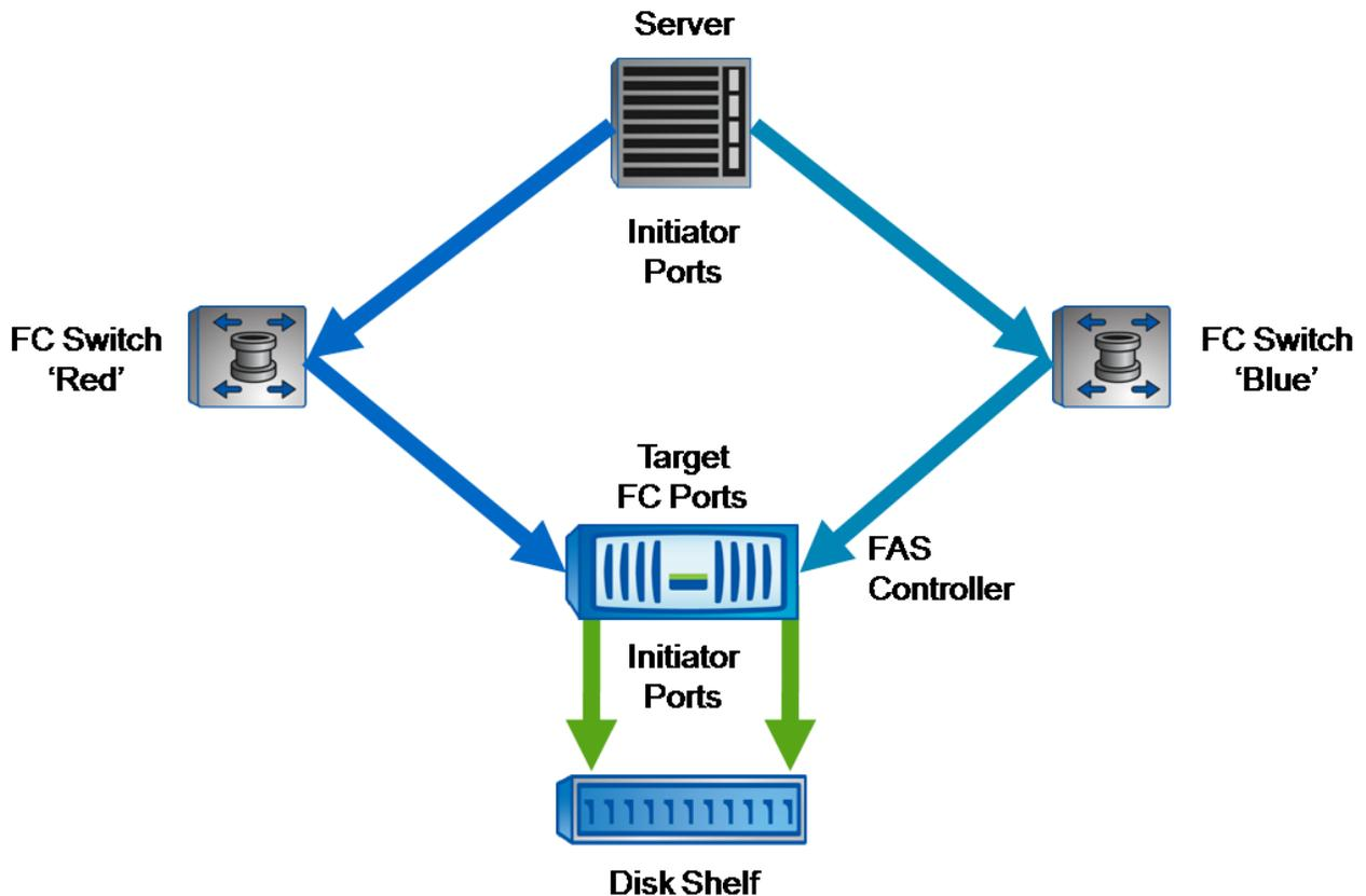
**FIGURE 4: FIBRE CHANNEL INITIATOR-TARGET PORT RELATIONSHIPS**
