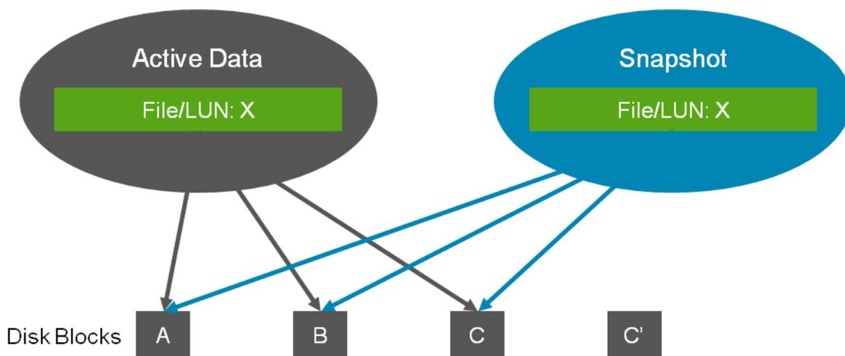
**FIGURE 16: THE PROCESS OF A SNAPSHOT COPY LOCKING SOME BLOCKS IN THE AFS**
